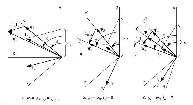
Fig. 2. Expedient and optimized regimes of synchronous motor:  $\mathbf{i}_s$  – representing vector of stator currents,  $\boldsymbol{\psi}_{\delta}$  – representing vector of main flux,  $\boldsymbol{\psi}_s$  – representing vector of stator flux linkages,  $\boldsymbol{\psi}_G$  – flux reference; d, q – axes of rotor,  $\rho$ ,  $\tau$  - axes connected with vector of main flux,  $\boldsymbol{\xi}_s$ ,  $\eta$  – axes connected with vector of stator flux
