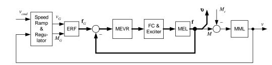
Fig. 1. Structural diagram of a synchronous drive control system: ERF – energy regimes former, MEVR – motor electromagnet variables regulator, MEL – motor electromagnet loops, MML – mechanical move link;  $\mathbf{f}$  – output vector of motor electromagnet loops,  $\mathbf{f} = (\mathbf{v}, M)$ ; references are designated with G subscript
